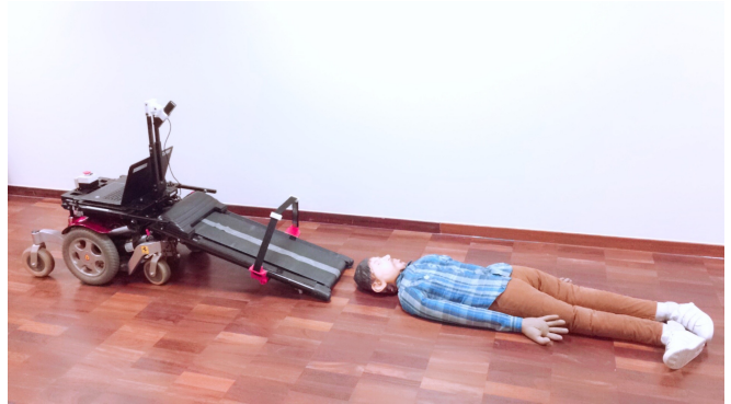
Fig. 1: Autonomous mobile rescue robot ResQbot [21] for casualty extraction scenarios. This platform comprises a motorised stretcher bed conveyor module attached to a differential-drive mobile base, a stretcher strap module and an RGB-D camera.
