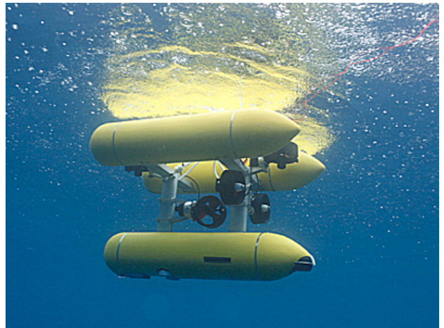
Fig. 1. The Girona 500 hover-capable AUV getting disturbed by waves at shallow depth in open water. A dynamic model of this AUV, obtained through system identification, is used for the simulated experiments described in this paper. [Photo credit: CIRIS Underwater Robotics Research Center, University of Girona, Spain]
