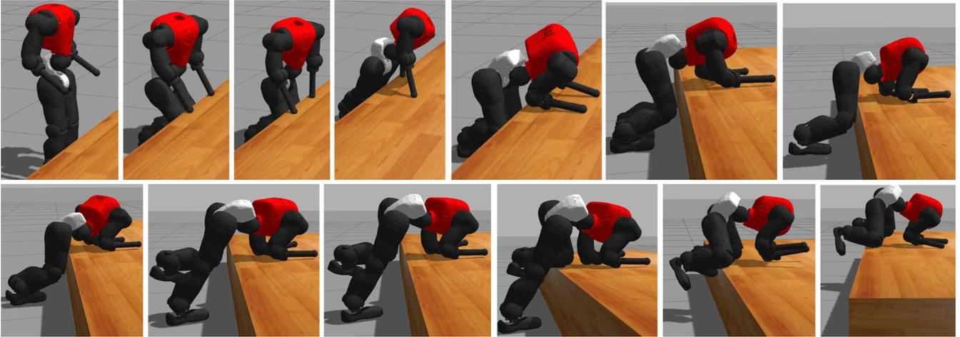
Fig. 6: This is a sequence of screenshots taken while the humanoid robot COMAN is climbing on top of the wooden obstacle in the simulated world.
