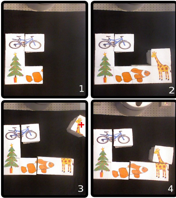
Fig. 9. Two operations during the demonstration phase by the caregiver in the domino task are shown in subfigures 1 and 2. Match detection result and the reproduced operation by the robot in the reproduction phase are shown in subfigures 3 and 4. The red cross on the object shows the detected positions for pick action by VSL. (details in section V-D).
