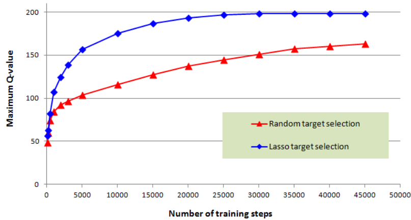
Fig. 12. Comparing Lasso target selection with Random target selection for Time Hopping. The maximum Q -value achieved relative to the number of training steps is used as an indicator of the ability of each selection method to discover early high-valued policies
