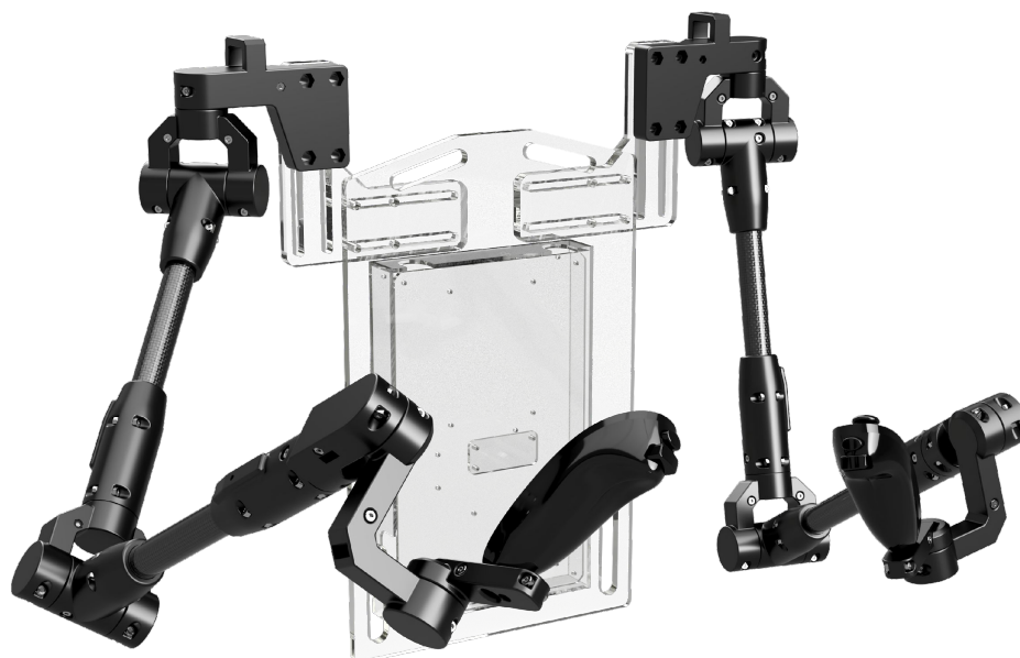
Figure 3. CAD model of the DE VITO, a dual-arm, upper-limb exoskeleton for semi-autonomous robot manipulation. Source: Falck et al. (2019)
