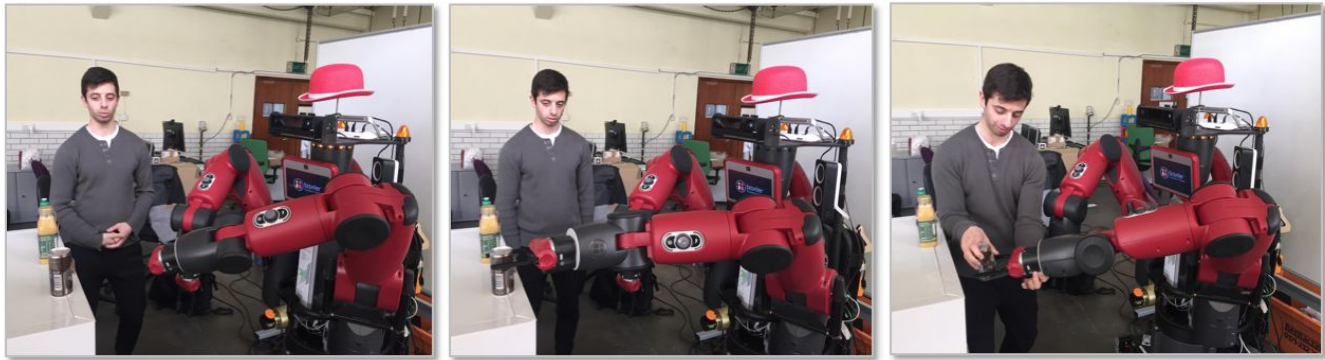
Figure 9. The three grasping stages of moving to an intermediate position (left), grasping the object (middle), and executing handover-mode (right). Written consent for using this figure by the person depicted has been obtained.
